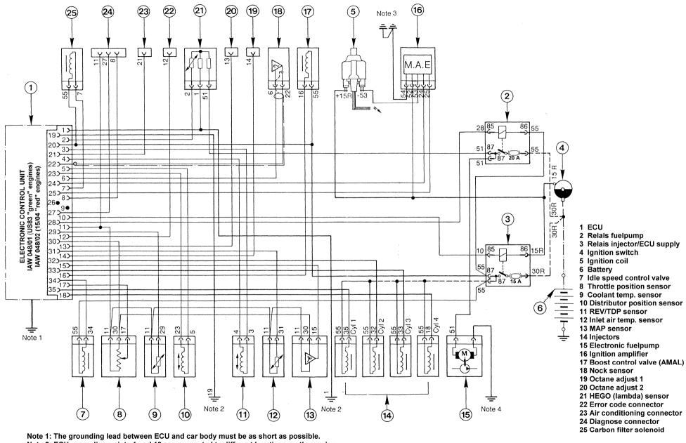
Note 2: ECU grounding points 1 and 19 are connected to different locations on the engine.
