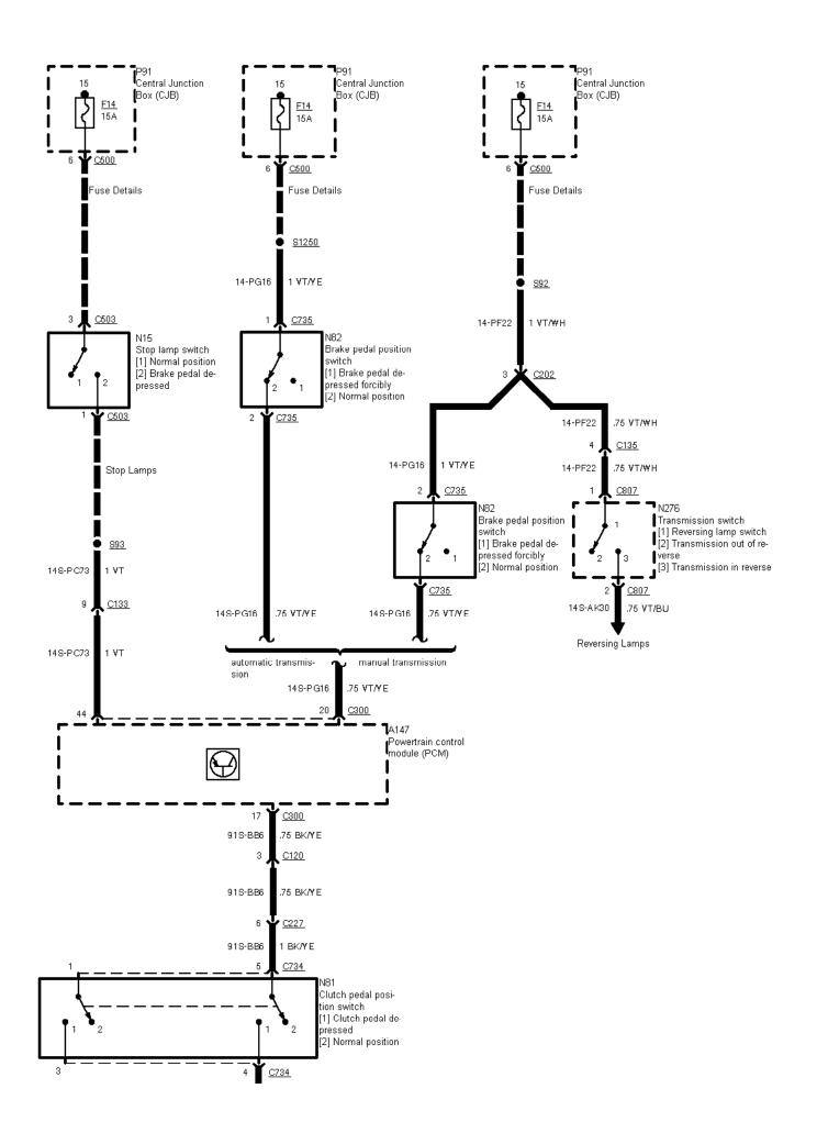
33-07-011, Speed Control, TCI Diesel automatic transmission
