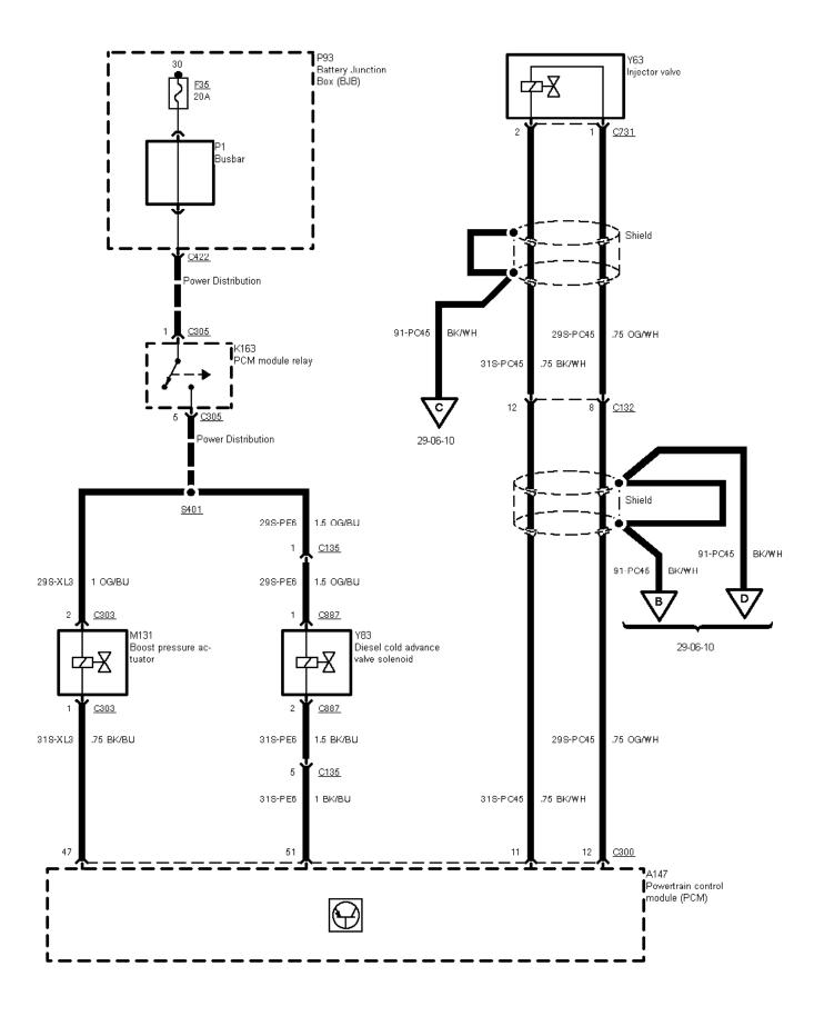
29-06-014 , Engine Control 2,5 I TCI Diesel (Manual Transmission) , As of 09/96
