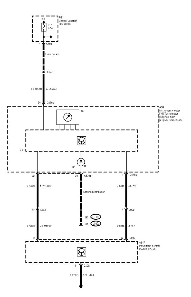
29-06-018 , Engine Control 2,5 I TCI Diesel (Manual Transmission) , As of 09/96, Pre-glow system
