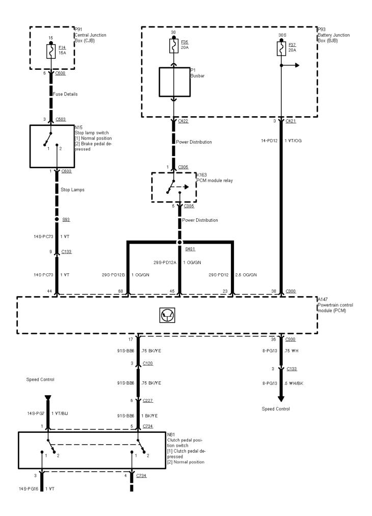
29-06-010 , Engine Control 2,5 I TCI Diesel (Manual Transmission) , As of 09/96
