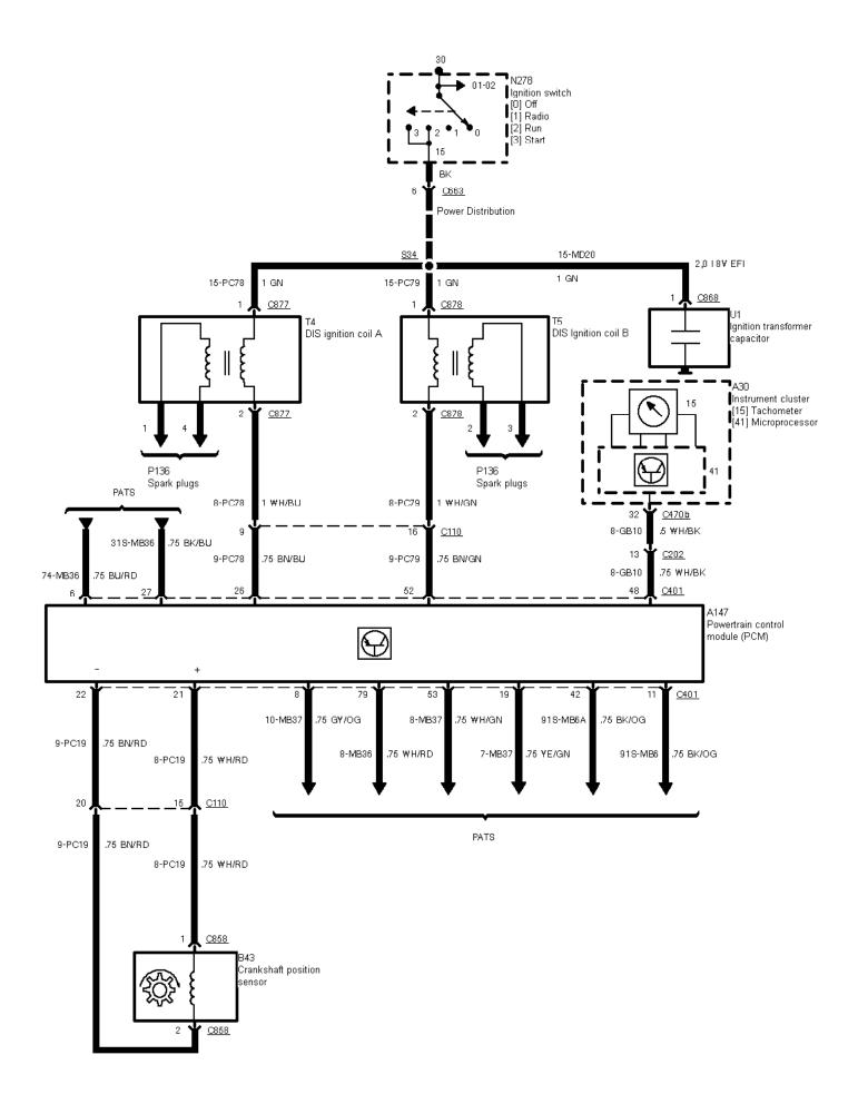
29-02-003 , Engine Control 2,0 I 8V/16V EFI (Manual Transmission) , Sensors
