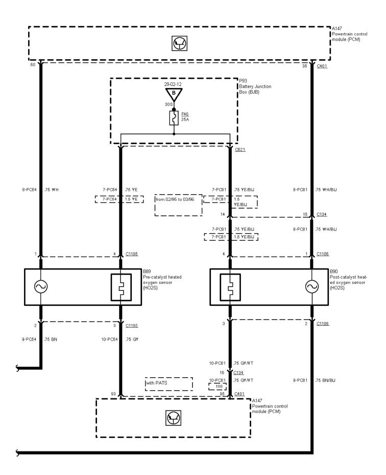
29-02-009, Engine Control 2,0 I 8V/16V EFI (Manual Transmission)
