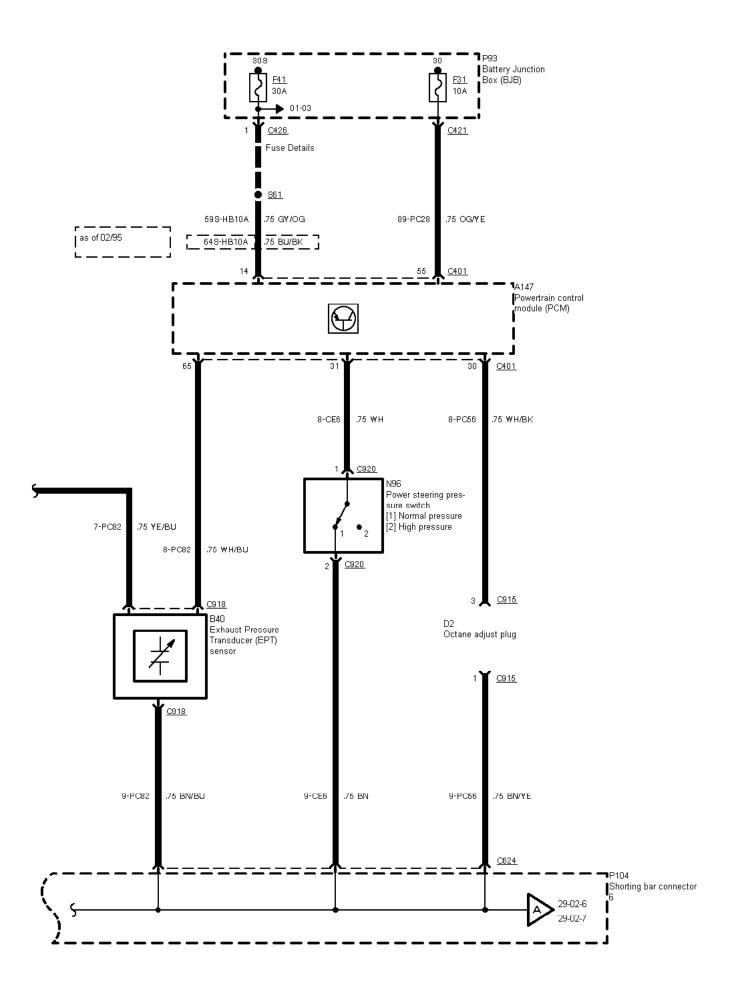
29-02-005, Engine Control 2,0 I 8V/16V EFI (Manual Transmission), Fuel injection
