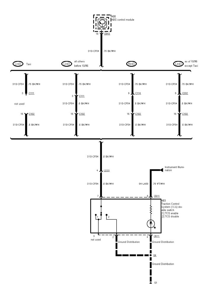
12-02-007 , ABS with Traction Control System (TCS) , Except 2,9 I V6  $12\mathrm{V}$
