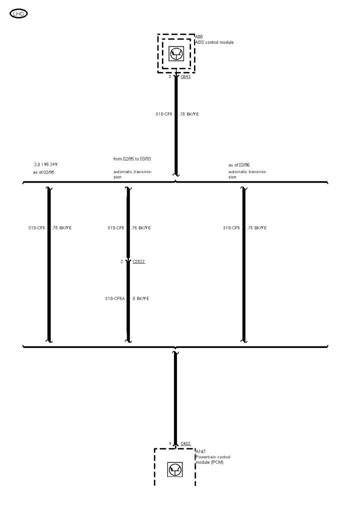
12-02-008 , ABS with Traction Control System (TCS) , Except 2,9 I V6 12V
