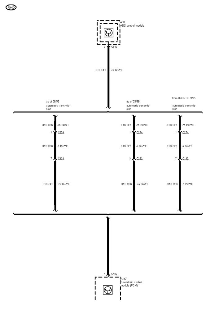
12-02-009, ABS with Traction Control System (TCS), Diagnostic connectors before 03/96
