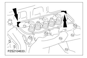
19. Coat the contact faces of the cylinder head cover flange with sealer (SPM-2G-3121-A).
