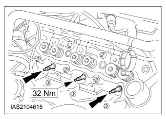
**NOTE:** Apply lubricant (Never Seez, ESE-M1244-A) to the spark plug threads.
