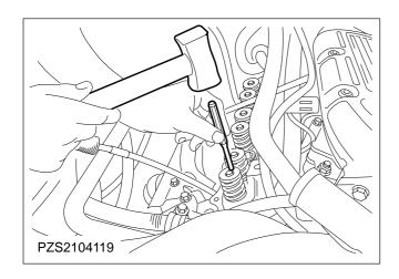
7. Release the valve collets by tapping on the valve heads.
