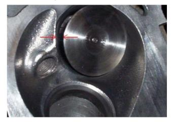
The valves themselves also need attention. There is a ridge in the back of each valve head, almost like a step. This needs to be considerably smoothed. Mounting the valve stem in the chuck of a drill and using emery paper on the valve head is an easy method of dealing with this.
