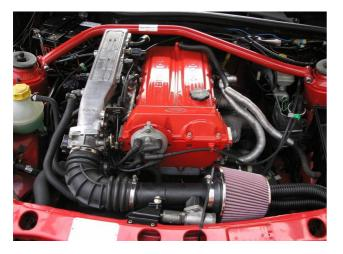
In terms of the intake manifold itself, it is fairly good with relatively long straight primaries leading into the side of the cylinder head.
