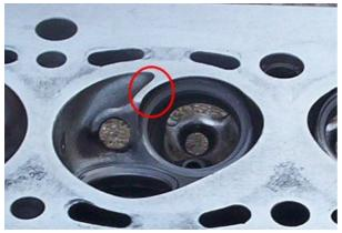
Because of this restriction, gains can be had by altering its shape to allow for more flow...
