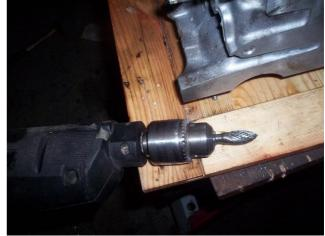
Drill-mounted carbide cutter – use carefully and do not attempt to remove too much material in one go!
