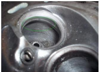
Step left in cylinder head by machining of valve seat (circled)
