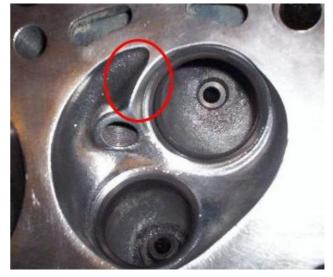
...by increasing the space for gas to pass through when the inlet valve is open.
