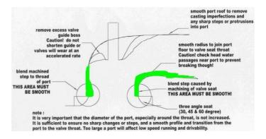
The biggest single area needing attention for both inlet and exhaust valves is the step left in the casting of the cylinder head by machining to fit the valve seat inserts. This can be seen in the following picture, circled in green:
