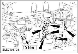
52. Fit the DIS ignition coils and the noise suppression capacitor.
