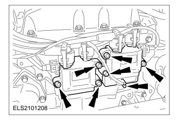
8. Remove the DIS ignition coils and the noise suppression capacitor.
