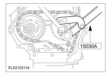
12. Release the camshaft sprockets.
