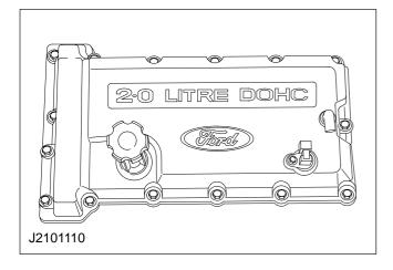
9. Remove the cylinder head cover (11 bolts, four nuts).
