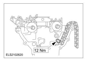
40. Tighten the chain guide rail.
