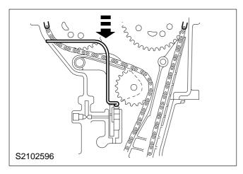
**NOTE:** If the hydraulic plunger does not reach the tensioning arm, unlatch the plunger with the aid of an auxiliary tool.
