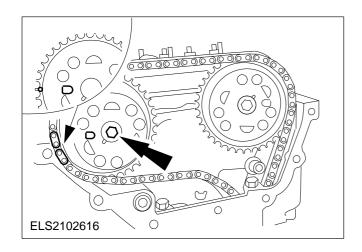
**NOTE:** It does not matter if the timing chain sags slightly between the sprockets.
