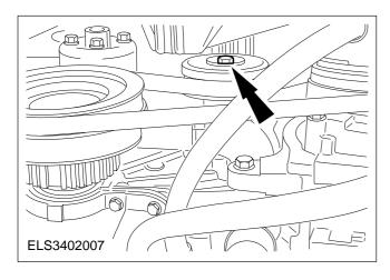
23. Release the tensioning pulley and remove the multi-groove belt.
