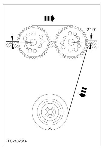
**NOTE:** If it is necessary to adjust the timing (and to loosen the chain) fit a new hydraulic plunger.
