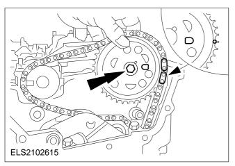
**NOTE:** The timing chain must be taut on the tensioned run.
