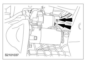
3. Remove the starter motor.
