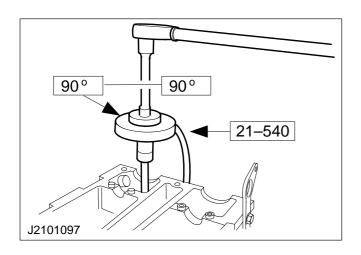
CAUTION: The cylinder head bolts must not be retorqued.
