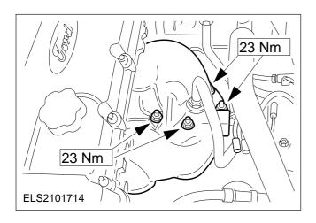
33. Attach the exhaust pipe to the exhaust manifold.
