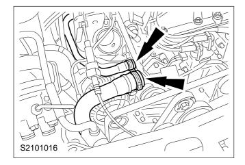
9. Disconnect the coolant hoses from the thermostat housing.
