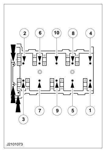
**NOTE:** Release the three auxiliary bolts first.
