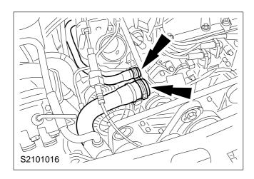
42. Attach the coolant hoses to the thermostat housing.
