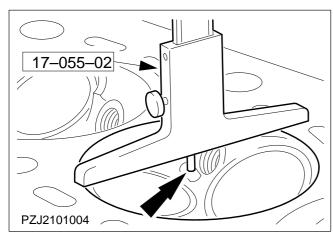
**NOTE:** Remove carbon deposits at the measuring site.
