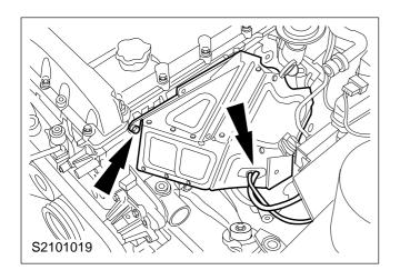
15. Detach the exhaust manifold heat shield (three bolts, one nut).
