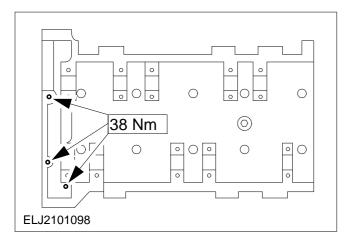
30. Tighten the auxiliary cylinder head bolts.
