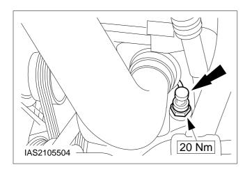
6. Fit the oil pressure switch and connect the oil pressure switch plug.
