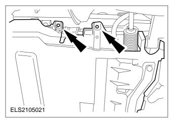
7. Attach the engine undershield (left-hand side shown).
