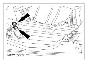
6. Remove the upper exhaust manifold nuts.
